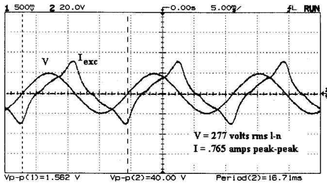
Fig. 4. Primary sinusoidal voltage and normal excitation current.
