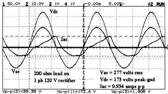
Fig. 5. Primary voltage and current and secondary diode voltage with half wave rectifier load on secondary.
