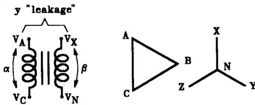
Fig. 1. Two-winding transformer showing node and branch voltages on one core.
