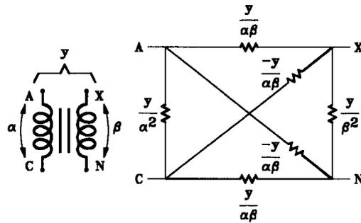
Fig. 2. Four-port admittance model of transformer.
