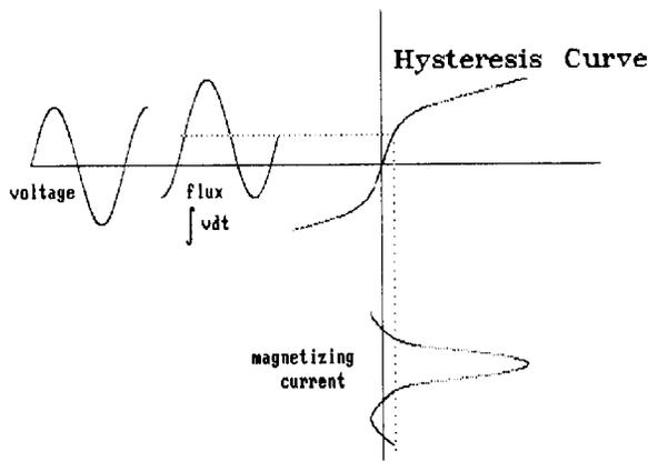
Fig. 3. Transformer flux offset due to dc load current.
