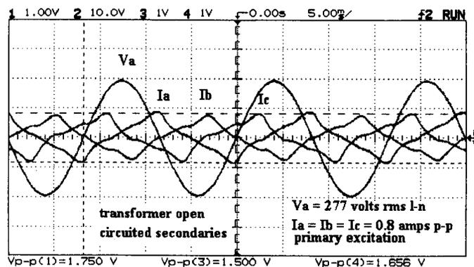
Fig. 6. Primary excitation currents and a phase voltage with all secondaries open circuited.
