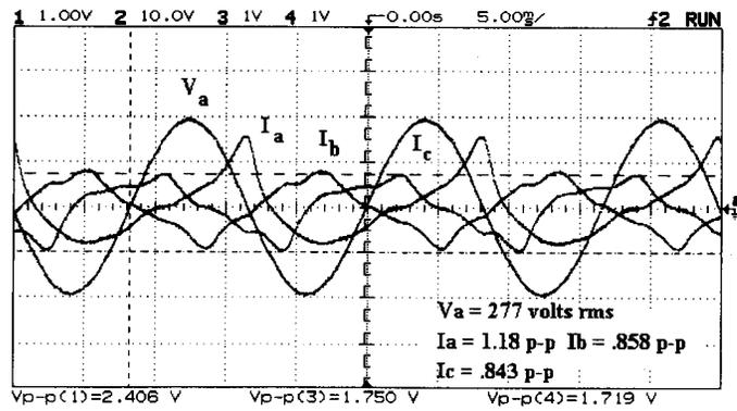
Fig. 7. Single-phase half wave rectifier on phase A causes distortion in primary current of all phases.
