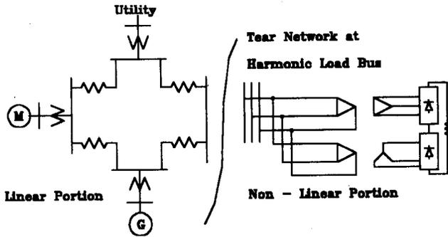
Fig. 8. Network torn into linear and nonlinear portions.
