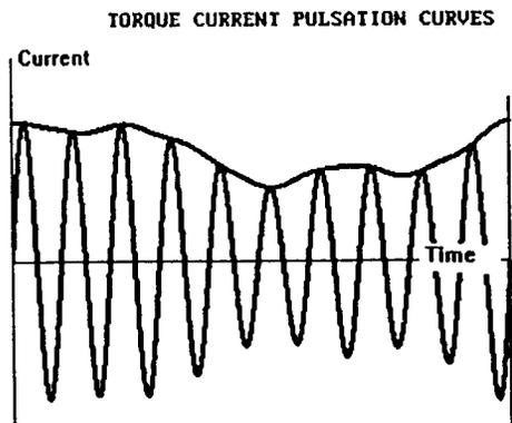
Figure 2 - Effect of Load Pulsation on Motor Current
