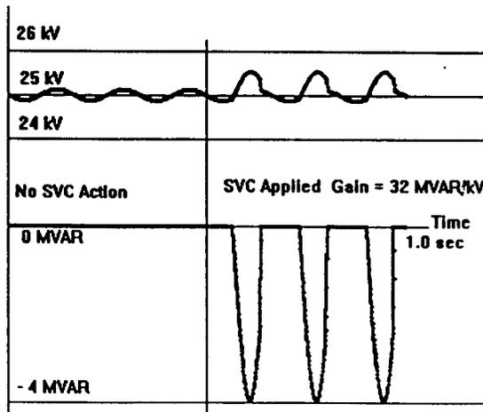
Figure 9 - Variation in Bus Voltage and SVC MVARs
