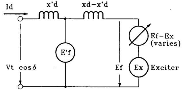
Figure 11 - Transient Equivalent Circuit
