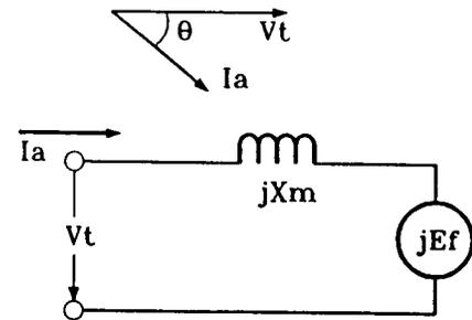
Figure 10 - Steady State Equivalent Circuit
