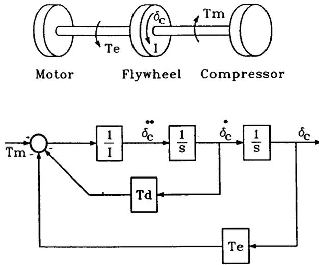
Figure 12 - Motor and Compressor Dynamic Model
