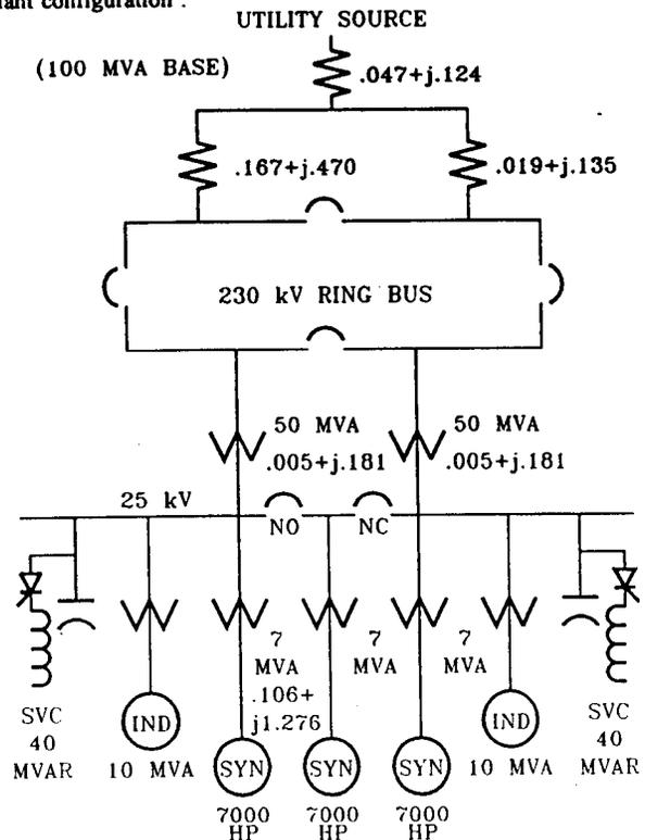
Fig. 1 - Plant Power Supply & Distribution
