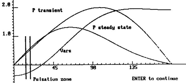
Fig. 5 - Motor Power Curves
