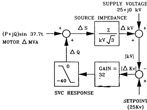
Figure 8 - SVC Interaction With The Motor
