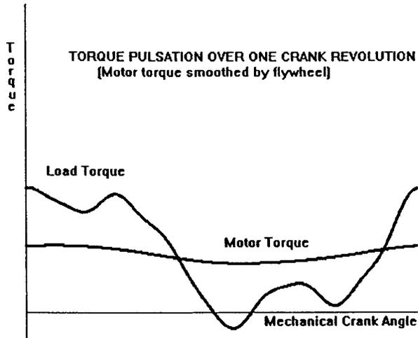
Fig. 4 - Torque Pulsation Versus Crank Angle
